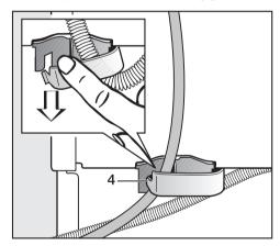
■ The lower clip (4) can be opened to allow you to take the drain hose out or to feed the mains cable through it.
